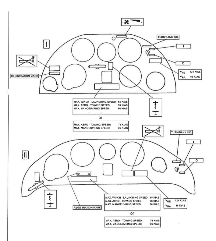
FIG. 3.7-4 INSIDE PLACARDS AND MARKINGS - FRONT AND AFT INSTRUMENT PANELS
